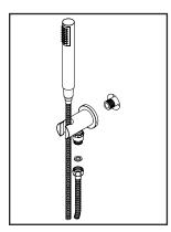
(1) Apply Teflon tape to the pipe nipple stretching out from the wall, attach drop ell with handheld support to pipe nipple. Install vacuum breaker to drop ell. Connect 60" stainless steel hose to vacuum breaker. Use silicone sealant to caulk around drop ell to create water tight seal. Turn on water and check for any leaks. Turn off water and connect handheld showerhead to 60' stainless steel hose.
