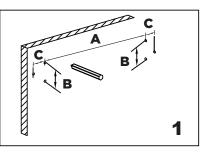
Mark (on the wall) locations of plugs through mounting plate using a pencil, refer to Fig.1
