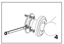
Driver bolt nut directly into holes
