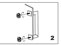
Screw in the fixing brackets into the handle bolts.
