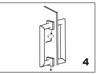
Fix the set screws on the end caps,tighten it to avoid loose from fixing brackets.
