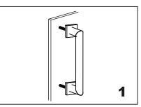
Install the handle A (bolt) through the glass holes,make sure the rubber gaskets are between handle&glass.
