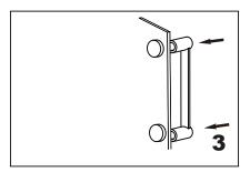
Add the handle A onto the fixing brackets, make sure the set screws holes in the bottom.
