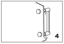
Fix the set screws on the handle A,tighten it to avoid loose from fixing brackets.
