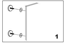
Install the end caps "4" (bolt) through the glass holes,make sure the rubber gaskets are between handle&glass.
