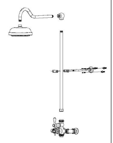
This faucet is tested to remain within 1 degree Fahrenheit of your desired setting throughout its operation, with an automatic temperature stop at 104 degrees Fahrenheit. The unit also has a built-in anti-syphon.
